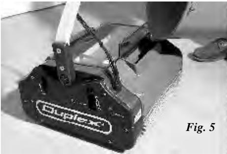
The tanks can be filled either by pouring water in from a jug, (fig. 5) or by placing the tanks themselves under a tap as they are easy to remove.
