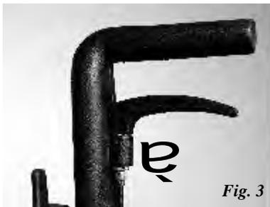
Adjust the screw of the register located underneath the lever of the handgrip, at the same time observing the positioning of the feelers that allow the liquid to exit from the tanks. (fig. 3)
