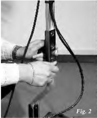
Assemble the handgrip if the handle by pushing it through the connecting casing and make sure to point the screws inwards with the cable-holder facing towards the bottom.
